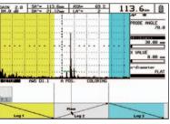
New "Color Leg" indicator displays the legs of the angle beam inspection in different colors
