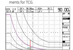
DAC Curve with 6 dB offset multiple curves
